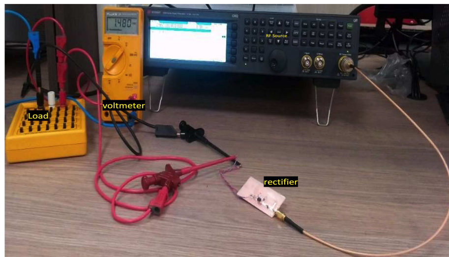
Figure 12. Lab-scale setup for measuring rectified voltage of PLA rectifier at 2.45 GHz while varying the load value.
