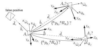
Fig. 1. Problem setting: robots (triangles) are shown with their attached frame and IMU measurements. Robot  $A_i$  detects two actual robots whose identities are unknown plus one false positive, resulting in three anonymous measurements.
