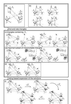
Fig. 3. Execution of P-MultiBeaReg3D in an ambiguous situation: (a) actual configuration (b) initial feature sets (c) triangle found in the first step containing the owner of the algorithm and their 2-intersections (d) maximal subset of irreconcilable triangles and their comparison with the current belief (e) other triangles found in the first step of the algorithm (f) expansion of the solution using the remaining triangles.
