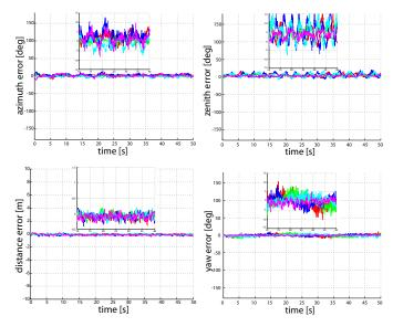
Fig. 5. Bearing+distance algorithm. Errors on azimuth, zenith-distance, distance and yaw estimates for  $A_2, \ldots, A_6$  computed by  $A_1$ , with a zoom for [10, 40] s.
