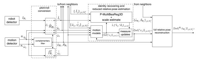
Fig. 2. Scheme of the mutual localization system that runs on the generic robot  $A_i$
