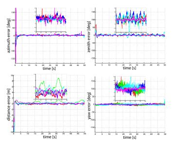
Fig. 4. Bearing-only algorithm. Errors on azimuth, zenithdistance, distance and yaw estimates for  $A_2, \ldots, A_6$ computed by  $A_1$ , with a zoom for [10, 40] s.
