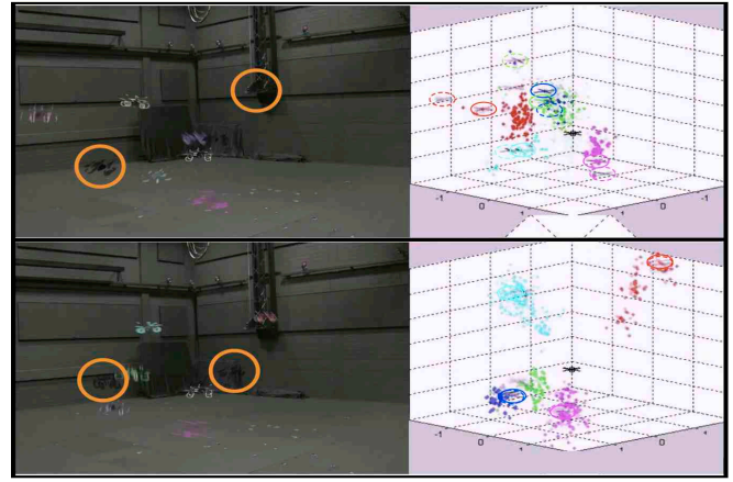
Fig. 9: Two snapshots from the first experiment. On the left, the scene as seen by a fixed camera; the circled quadrotors act as false positives and do not communicate with the others. On the right, the estimates computed by the filters at the same time instants. The dots represent the best 100 particles. For each quadrotor, the solid circled cross represents the best particle, while the dashed circled cross represents the ground truth. The first snapshot is taken at the very beginning of the experiment, while in the second snapshot the relative distances among the robots have already been retrieved.
