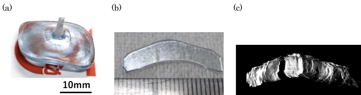
Fig. 2. (a) picture of grown crystal, (b) cross sectional picture and (c) X-ray topography of the same sample.
