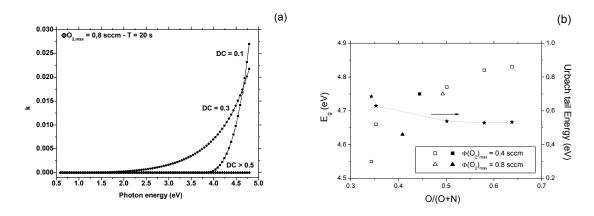
Figure 6: (a) Extinction coefficient as function of photon energy for  $\Phi_{max}(O_2) = 0.8$  sccm, T = 20 s and various DC, and (b) Optical bandgap for various pulse conditions, T = 20 s (open) and T = 40 s (full), and Urbach tail energy for  $\Phi_{max}(O_2) = 0.4$  sccm, T = 20 s.
