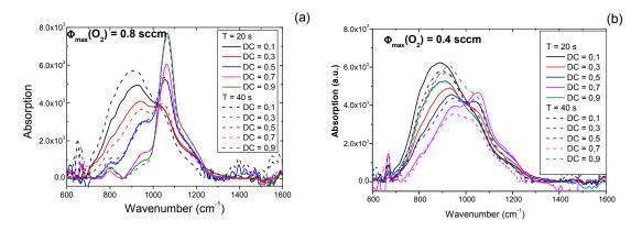
Figure 3: IR spectra for films deposited in PP with various duty cycles, for T=20~s (full line) and T=40~s (dash line), for (a)  $\Phi_{max}(O_2)=0.8~scm$  and (b)  $\Phi_{max}(O_2)=0.4~scm$ .
