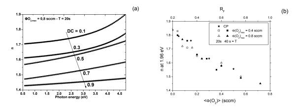
Figure 5: (a) Refractive index as function of wavelength for  $\Phi_{max}(O_2)=0.8$  sccm, T=20 and various DC, and (b) refractive index at 1.96 eV as function of  $R_F$  (top axis) and  $<\Phi_{O2}>$  (bottom axis) for films deposited in CP and PP respectively.
