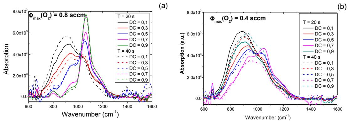
Figure 3: IR spectra for films deposited in PP with various duty cycles, for  $T = 20$  s (full line) and  $T = 40$  s (dash line), for (a)  $\Phi_{\max}(\text{O}_2) = 0.8$  sccm and (b)  $\Phi_{\max}(\text{O}_2) = 0.4$  sccm.
