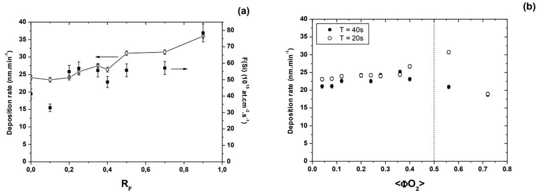
**Figure 2: (a) Deposition rates (open) and incorporated silicon flux (full) calculated in CP and, (b) deposition rates in PP for both periods  $T = 20$  (open) and 40 s (full).**
