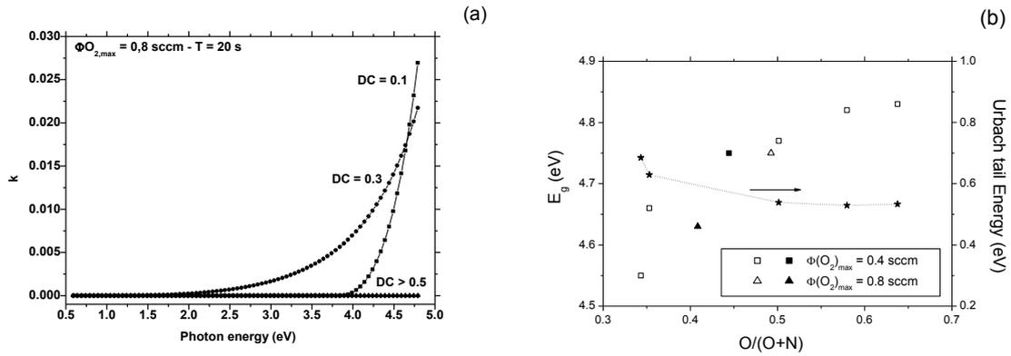
**Figure 6:** (a) Extinction coefficient as function of photon energy for  $\Phi_{\max}(\text{O}_2) = 0.8$  sccm,  $T = 20$  s and various DC, and (b) Optical bandgap for various pulse conditions,  $T = 20$  s (open) and  $T = 40$  s (full), and Urbach tail energy for  $\Phi_{\max}(\text{O}_2) = 0.4$  sccm,  $T = 20$  s.
