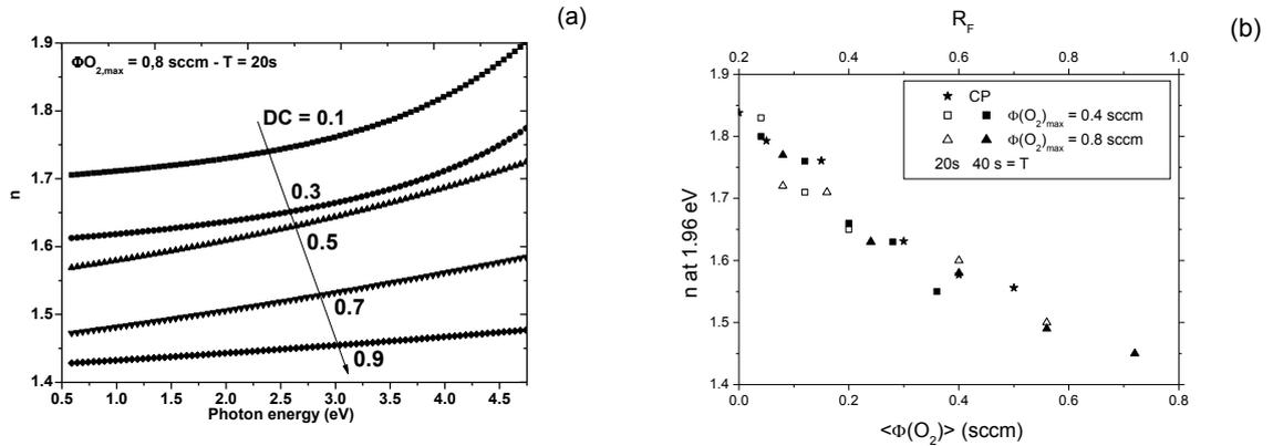
**Figure 5:** (a) Refractive index as function of wavelength for  $\Phi_{\text{max}}(\text{O}_2) = 0.8$  sccm,  $T = 20$  and various DC, and (b) refractive index at  $1.96\text{ eV}$  as function of  $R_F$  (top axis) and  $\langle\Phi_{O_2}\rangle$  (bottom axis) for films deposited in CP and PP respectively.
