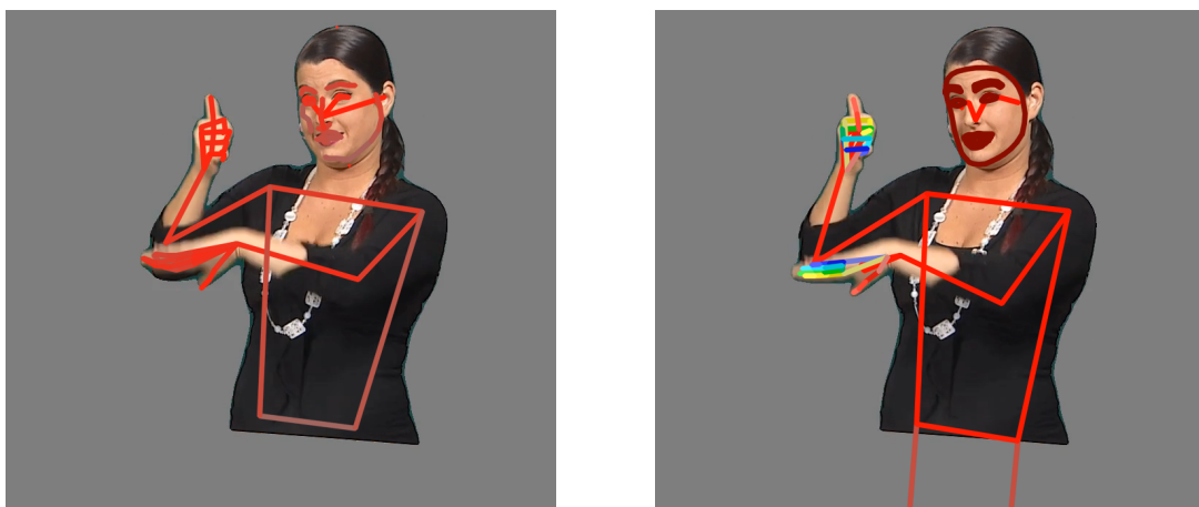
Figure 2: Examples of the output of pose estimation systems overlaid over the original video frames. Left: OpenPose, right: MediaPipe Holistic. Taken from Müller et al. (2022).
