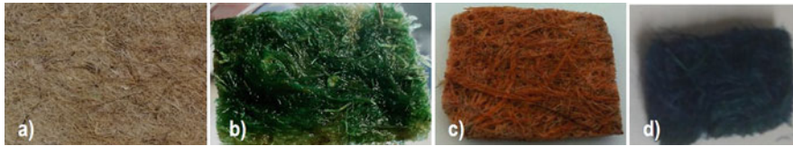
Fig. 5 Hemp before (a) and after biosorption in a solution containing copper (b), cobalt (c) or blue dye (d). Copyright G. Crini
