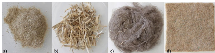
Fig. 3 Different forms of hemp-based materials: (a) powders, (b) shives or hurds, (c) fibers and (d) felt. Copyright G. Crini
