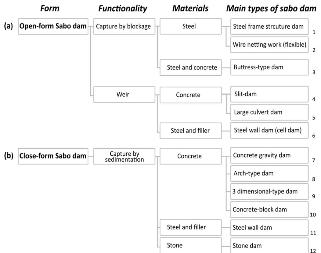
**Figure 5.** Sabo dam classification according to the MLIT documents [29]. (a,b) MLIT classified twelve main types of Sabo dams regarding their form, functionality, and materials. They are the main types of Sabo dam we can find in the construction projects. Translated and modified by Mélody Dumont.
