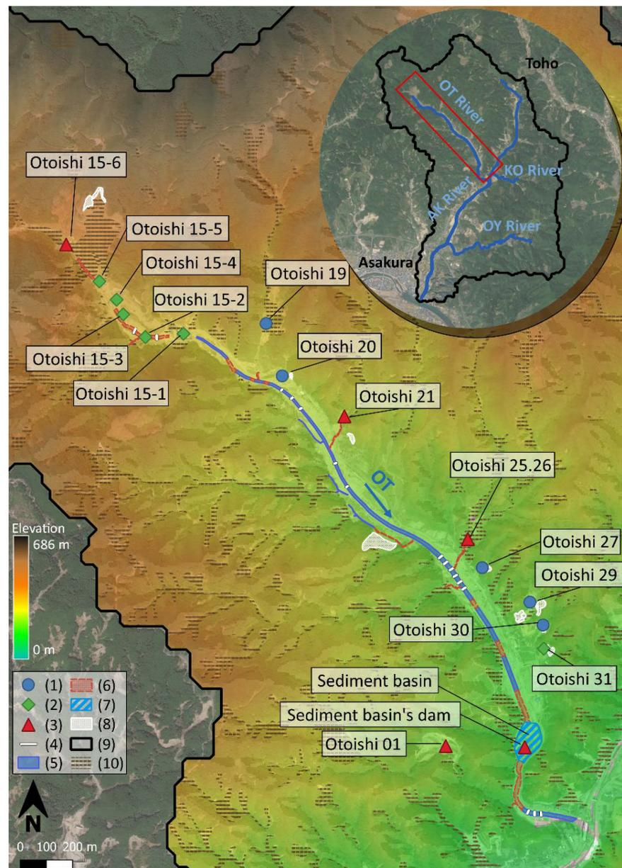
**Figure 10.** Sabo works' organization in the Otoishi River. (1) semi-open form Sabo dam; (2) closed-form Sabo dam; (3) open-form Sabo dam; (4) weir; (5) constructed canal; (6) canal under construction; (7) sediment deposit area; (8) hillside work; (9) watershed boundaries; (10) 2017 landslides [18].
