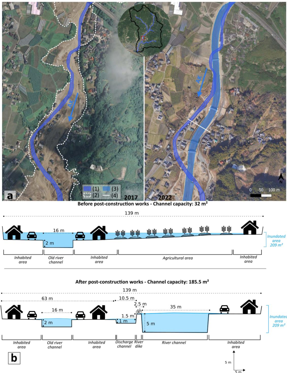
**Figure 9.** (a) Example of reconstructed channel damaged after J17 hydro-gravity hazards. (1) 2009 channel; (2) 2017's flood area; (3) 2022 channel, (4) river cross-section area. (b) river cross-section done during the 2023 field mission.
