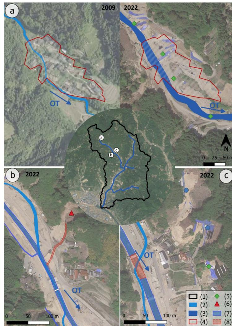
**Figure 11.** Close-ups of the OT watershed. (a). Evolution of the Otoishi hamlet before the disaster and during the reconstruction process. (b). Close-up of Sabo #21. (c). Close-up of Sabo #29, #30, #31. (1) Watershed boundaries; (2) 2009 river; (3) 2022 river; (4) OT hamlet; (5) open-form Sabo dam; (6) closed-form Sabo dam; (7) constructed channel; (8) channel under construction.
