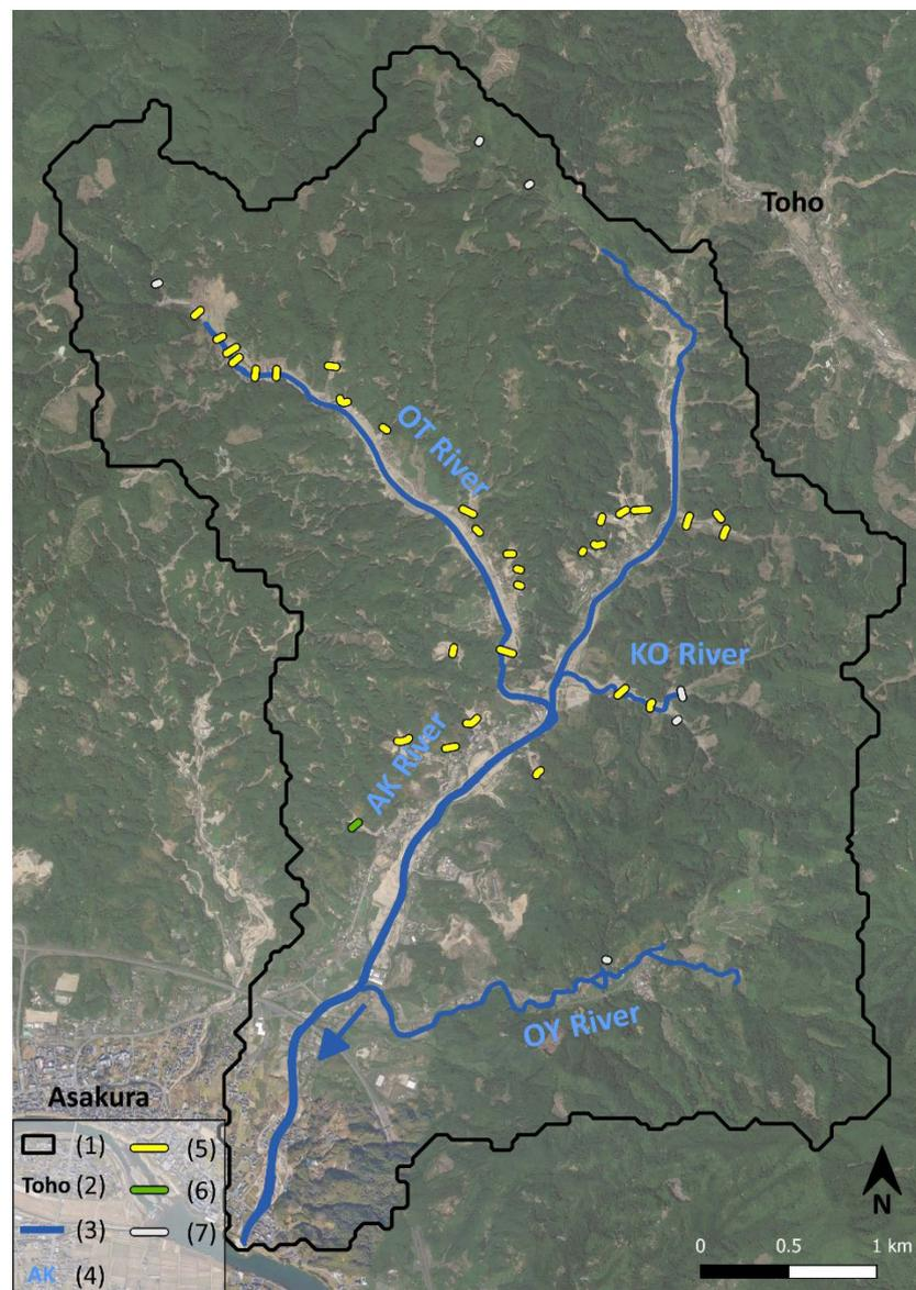
**Figure 8.** Location of Sabo dams in the Akatani watershed. (1) watershed boundaries; (2) toponyms; (3) river channels; (4) hydronyms; (5) Sabo dams constructed by the MLIT after 2017; (6) Sabo dams constructed by the prefecture after 2017; (7) Sabo dams constructed by the prefecture before 2017.
