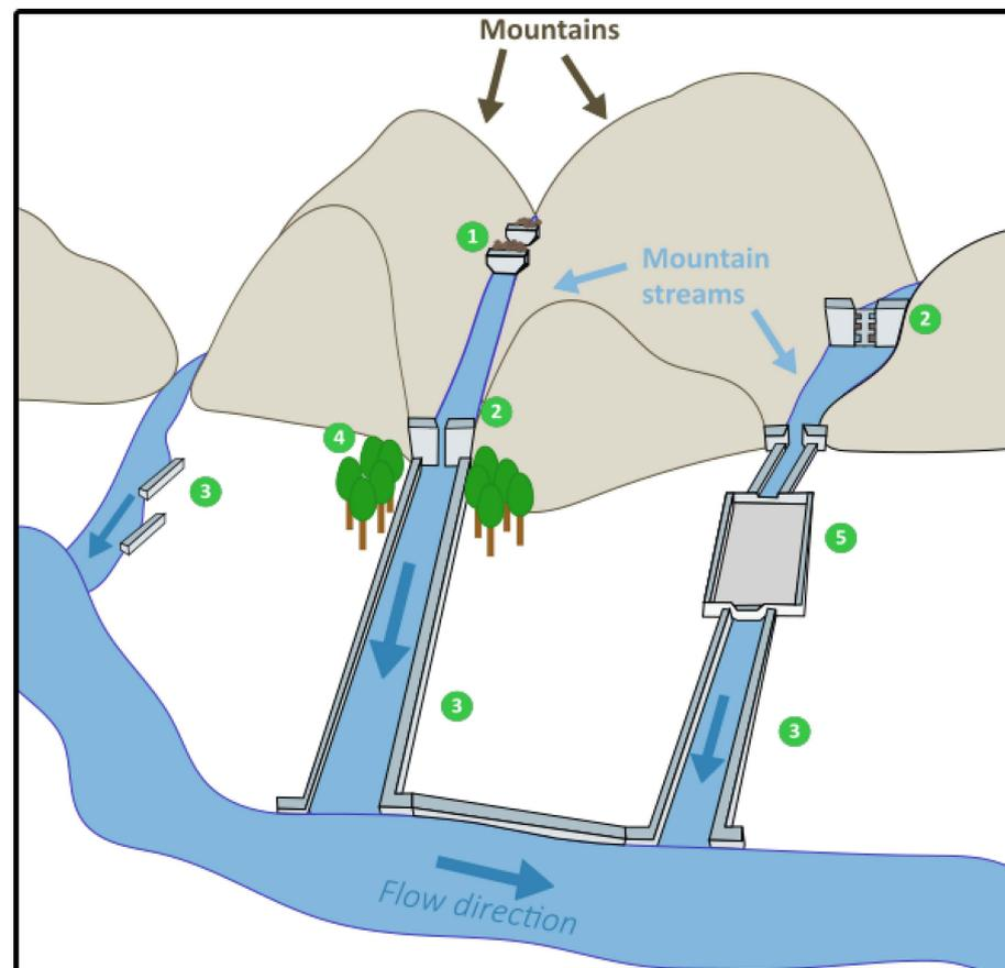
**Figure 4.** Example of Sabo built to mitigate the impact of debris flows. Modified according to Okubo et al. [30]. (1) occurrence controlling works; (2) capturing works; (3) controlling flow direction; (4) dispersion work; (5) depositing area works.
