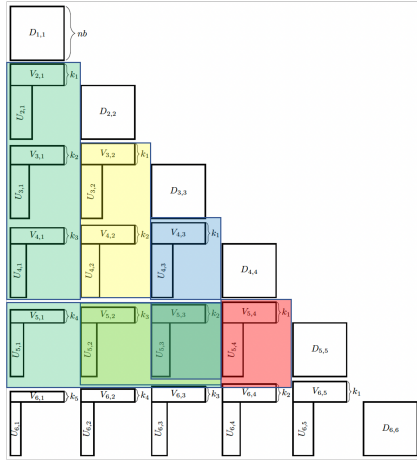
Fig. 9: Tile low-rank Cholesky factorization powered by a batch GEMM for climate applications.
