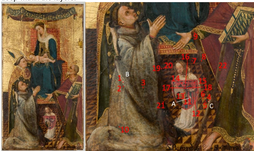
Fig. 1 a) Photograph of the painting Virgin and Child surrounded by saints and a donor (RFML.PE.2018.51.1). © C2RMF, T. Clot and b) detail showing the locations where the three cross-sections were taken in white (A, B and C), and in red the 22 locations where CXRF depth profiles were applied
