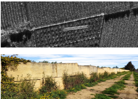
Fig. 1: A rotated double bounce signature in a SAR image, Top : X-band SLC image. Bottom : ground observation.
