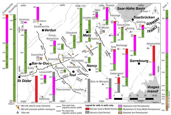
**Figure 3.** Location of studied seismic profiles and synthetic well data of the Permo-Carboniferous successions in the Lorraine Basin. Wells including velocity survey and synthetic seismogram are reported with colored triangles (see legend). Synthetic seismograms in Gironville and Francheville wells are presented in Figure 4.
