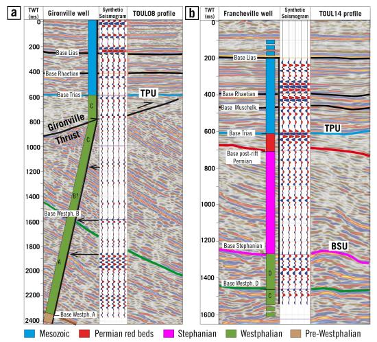
**Figure 4.** Seismic-well tie (a) between the Gironville well and the TOUL08 seismic profiles, and (b) between the Francheville well and the TOUL14 seismic profile. The Gironville well is the only well reaching the base of the Westphalian succession in Lorraine. The Francheville well traverses the Base Stephanian Unconformity (BSU).
