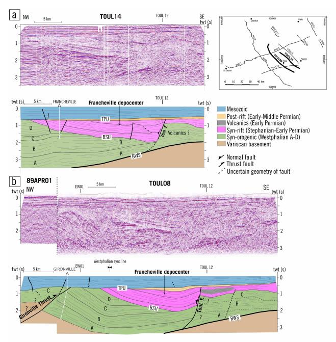
**Figure 6.** Reprocessed transverse seismic profiles (a) TOUL14 and (b) 89APR01-TOUL08; uninterpreted and interpreted. These profiles clearly emphasize the Base Stephanian Unconformity (BSU). Note also the maximum thickness of the synrift depocenter (Stephanian-Early Permian) onto the most deeply eroded part of the folded Westphalian succession thereby featuring a major topographic and tectonic inversion process.
