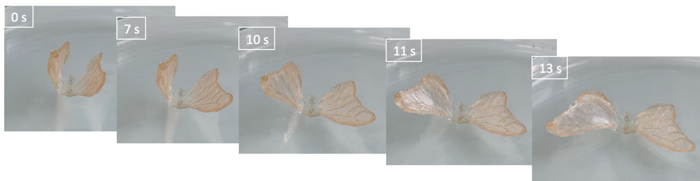
Figure 7. Movement of butterfly wings in heating (e.g. P(EHMA 20 - co -CoumMA 80 )).
