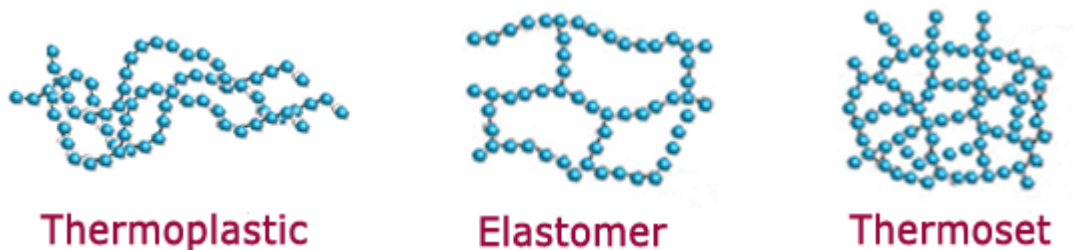
Figure 2. Different shapes of molecular chains of thermoplastic, elastomer and thermoset. Reproduced with permission from Wiley. 27
