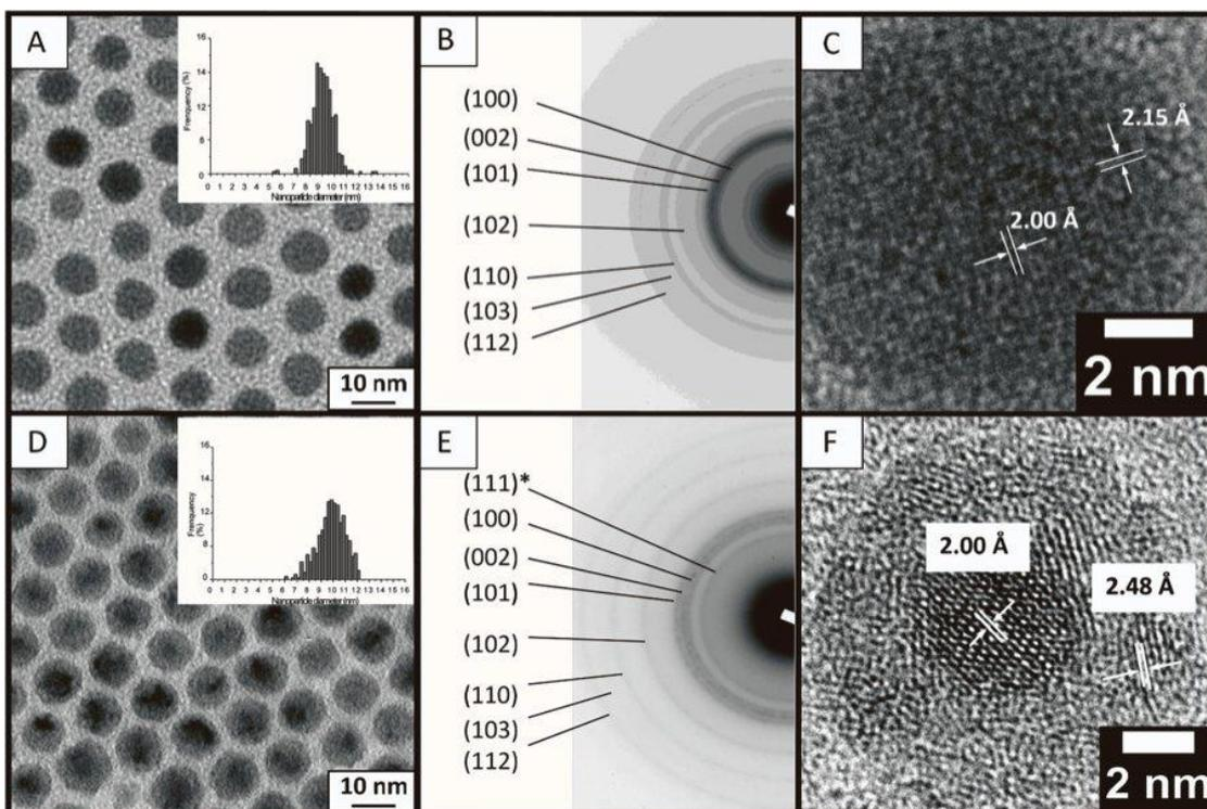
**Figure 3.** (A) TEM image of 9.0 nm Co hcp nanoparticles, (B) corresponding electron diffraction pattern and (C) HRTEM image of a single nanoparticle. (D) TEM image of 9.9 nm Co<sub>hcp</sub>@CoO nanoparticles, (E) corresponding electron diffraction pattern and (F) HRTEM image of a single nanoparticle.
