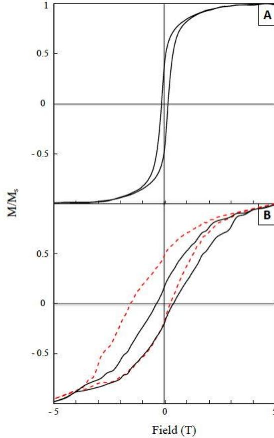
**Figure 5.** Hysteresis curves taken at 3K of (A) Co hcp nanoparticles (solid line) and (B)  $\text{Co}_{\text{hcp}}@ \text{CoO}$  nanoparticles in ZFC mode (solid line) and FC mode (dashed line).
