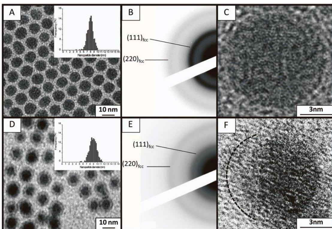
**Figure 2.** (A) TEM image of 7.9 nm Co fcc nanoparticles, (B) corresponding electron diffraction pattern and (C) HRTEM image of a single nanoparticle. (D) TEM image of 8.8 nm  $\text{Co}_{\text{fcc}}@\text{CoO}$  nanoparticles, (E) corresponding electron diffraction pattern and (F) HRTEM image of a single nanoparticle.
