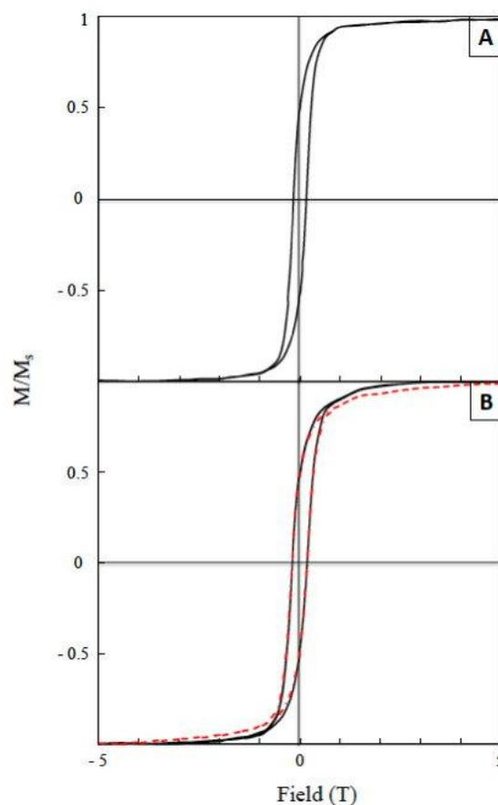
**Figure 4.** Hysteresis curves taken at 3K of (A) Co fcc nanoparticles (solid line) and (B) Co<sub>fcc</sub>@CoO nanoparticles in ZFC mode (solid line) and FC mode (dashed line).
