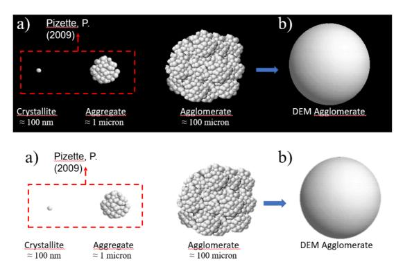
Figure 2 – a) Crystallite, aggregate, and agglomerate length scales for DEM simulations (P. Pizette [16]). b) An agglomerate represented by a single DEM sphere used here.
