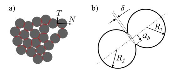
Figure 1 – a) Sketch of a discrete medium simulated by DEM with contact forces with normal (N) and tangential (T) components. b) Two DEM particles of radius  $R_i$  and  $R_j$  indented (indentation  $\delta$ ) and forming a bond of size  $a_b$ .
