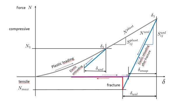
Figure 3 – Evolution of a contact between two agglomerates using an elastoplastic model. A contact may be plastic if the overlap increases through time and is irreversible or elastic if unloading arises. A contact may snap if this overlap decreases further than a critical value. Note how the unloading stiffness increases as the plastic indentation increases.
