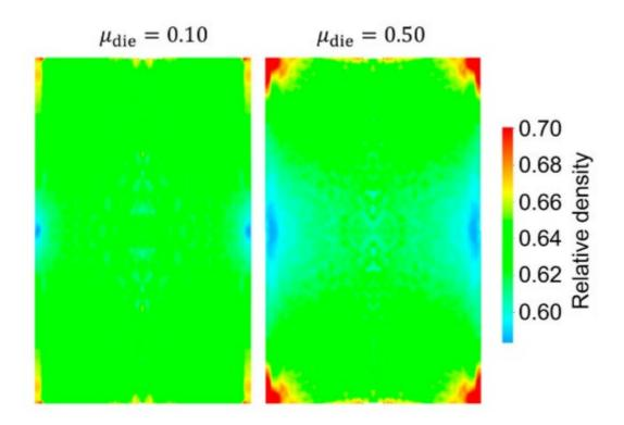
Figure 8-2D density gradient of a 3D compact: influence of the friction coefficient between agglomerates and the cylinder die  $\mu_{die}$ .
