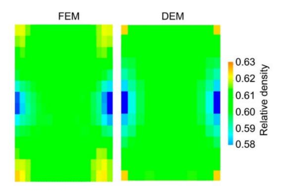
Figure 7 – Density gradient of the pellet cross-section after loading for FEM (adapted from [23]) and DEM simulations.
