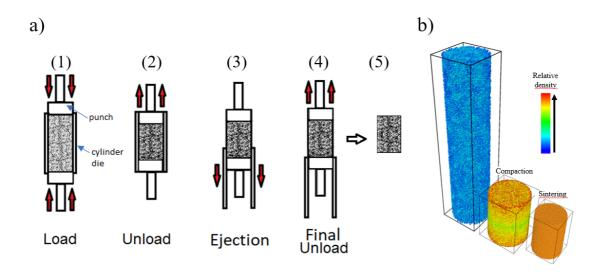
Figure 4 - a) Process kinematics of the compaction process implemented for DEM simulations, b) DEM compact before compaction, after compaction and after sintering.
