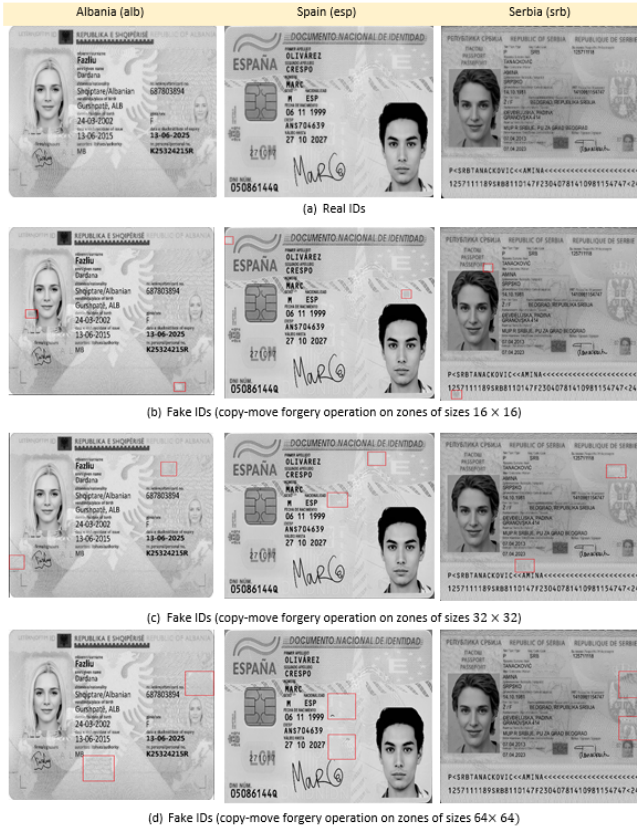
Fig. 2: Sample of MIDV and FMIDV: (a) real samples of three different countries, (b-d) fake samples of the three real IDs after applying copy-move forgeries with different zone sizes; red boxes present the forgery locations.
