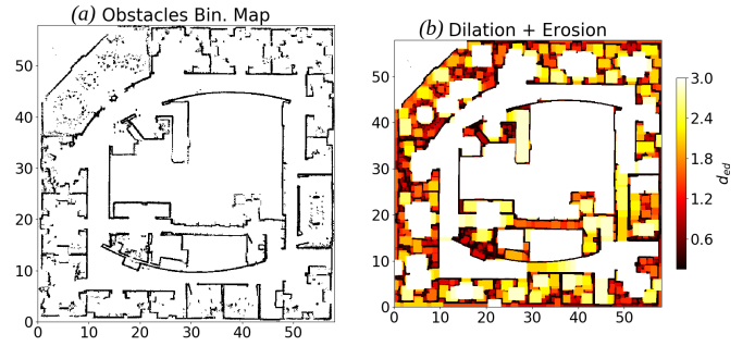
Fig. 2: Occupancy preprocessing - left: binary obstacles map, right: filtered obstacles obtained for various values of the d_{ed} parameter (obstacles dilation and erosion distance). Note: All units on the figures representing 2D maps are in meters.
