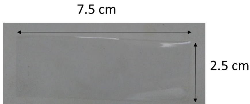
Figure S1: Photo of 87 – 90% hydrolysed PVA film before stretching. Film forming solution: 10 wt% PVA powder and 2 wt% glycerol.
