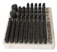
Fig 4: BPY specimens on an amorphous silica substrate (50x50mm<sup>2</sup>) manufactured by selective laser melting
