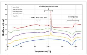
Fig 2: DTA curves of various crystalline and amorphous powder mixtures of Pic d'Ysson basalt (BPY) analog (wt.%), during first heating. To facilitate the readability of the graph, the curves have been translated vertically to avoid overlapping
