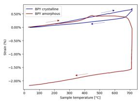
Fig 3: TMA curves of Pic d'Ysson basalt (BPY) analog during a first thermal cycle, with a 20 hr isothermal dwell at 720°C.
