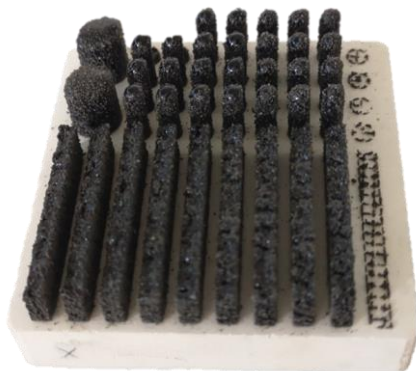
Fig 4: BPY specimens on an amorphous silica substrate (50x50mm 2 ) manufactured by selective laser melting
