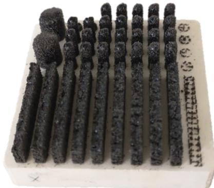
Fig 4: BPY specimens on an amorphous silica substrate (50x50mm<sup>2</sup>) manufactured by selective laser melting
