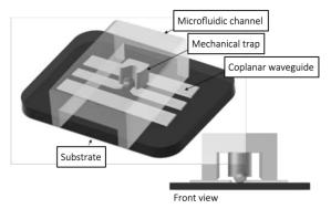
**Figure 1**: Schematics of the microdevice used for single cell EP and analysis [3].
