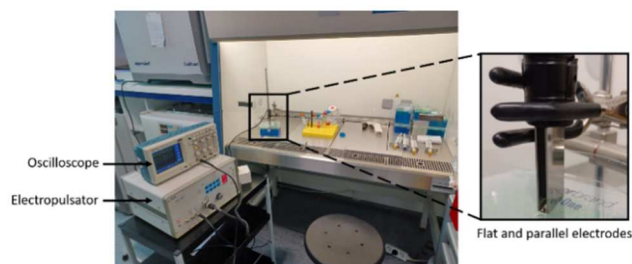
Fig 2 – Test bench for performing EP or ECT treatments on HCT-116 cells in suspension. The test bench includes an electropulsator to which an oscilloscope and electrodes are connected.
