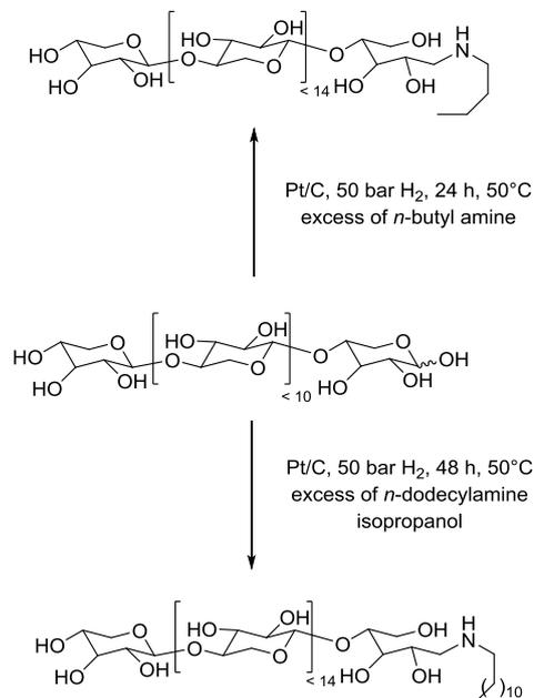
Figure 6. Pt/C-catalyzed reductive amination XOS with *n*-alkylamines. For the sake of clarity, only linear structures of XOS are shown.
