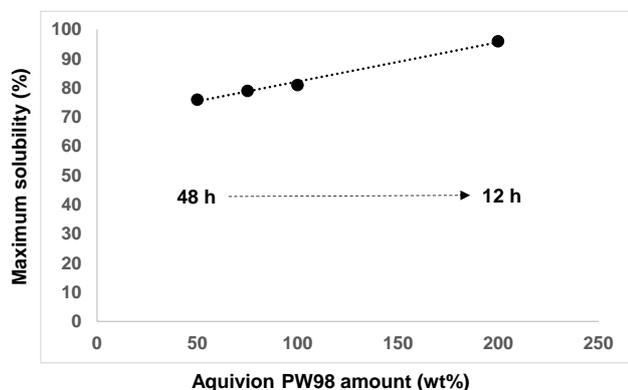
Figure 5. Effect of the Aquivion PW98 amount (wt%) on the maximum yield of water soluble XOS.
