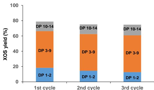
Figure 3. catalyst recycling using Pulp-HEM with 3.5 wt% of water
