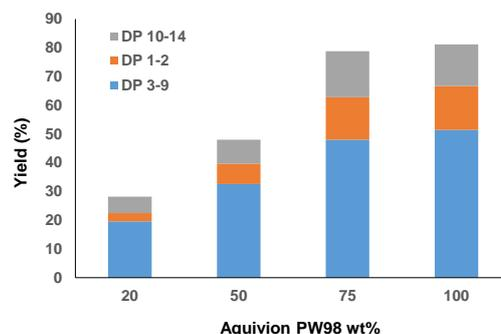
Figure 4. Effect of the Aquivion PW98 amount (wt%) as a function of Pulp-HEM solubility in water after 12 h of mechanocatalytic depolymerization.
