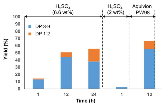
Figure 1. Mechanocatalytic depolymerization of Pine-HEM as a function of time, H<sub>2</sub>SO<sub>4</sub> amount and catalyst nature
