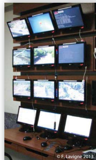
Webcam monitoring system for lahar observation at BPPTK and Balai Sabo
