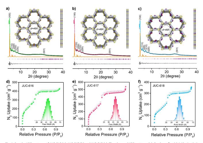
**Fig. 1.** Powder XRD patterns of JUC-616 (a), JUC-617 (b) and JUC-618 (c). The observed XRD patterns (+), Pawley refined (pink), simulation (orange), the difference between the observed and refined profiles (black) and Bragg position (green). Insets: crystal structures with AA stacking modes. Nitrogen adsorption (filled circles)-desorption (open circles) isotherms of JUC-616 (d), JUC-617 (e) and JUC-618 (f). Insets: pore size estimated using non-local density functional theory.
