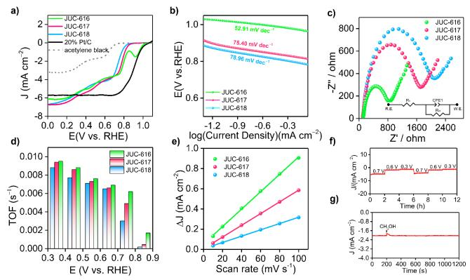
Fig. 2. (a) LSV curves of three isomorphic COFs in  $O_2$ -saturated 0.1 M KOH electrolyte at a scan rate of 1600 rpm. (b) Tafel plots of three COFs. (c) The impedance of COFs at open circuit voltage. Inset: equivalent circuit. (d) TOFs and mass activities of COFs. (e) Cdl values of COFs. (f) Multi-step amperometry curve of JUC-616 at an applied voltage of 0.3, 0.6 and 0.7 V. (g) Current-time curve of JUC-616 at 0.7 V vs RHE.
