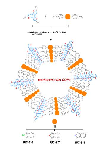
**Scheme 1.** Synthesis and chemical structures of isomorphic BTT-COFs (JUC-616, JUC-617, and JUC-618).
