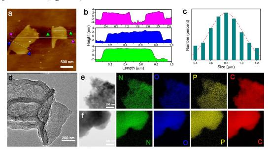
**Fig. 2 a** AFM image of JUC-610-CON, and **b** the corresponding height curves for the selective areas in **a**. **c** Lateral size distribution histogram of JUC-610-CON, and Gaussian fit curve is colored in red. **d** TEM image of JUC-610-CON. **e** and **f** TEM and the related elemental mapping images of carbon, nitrogen, oxygen, and phosphorus for JUC-610 and JUC-611.
