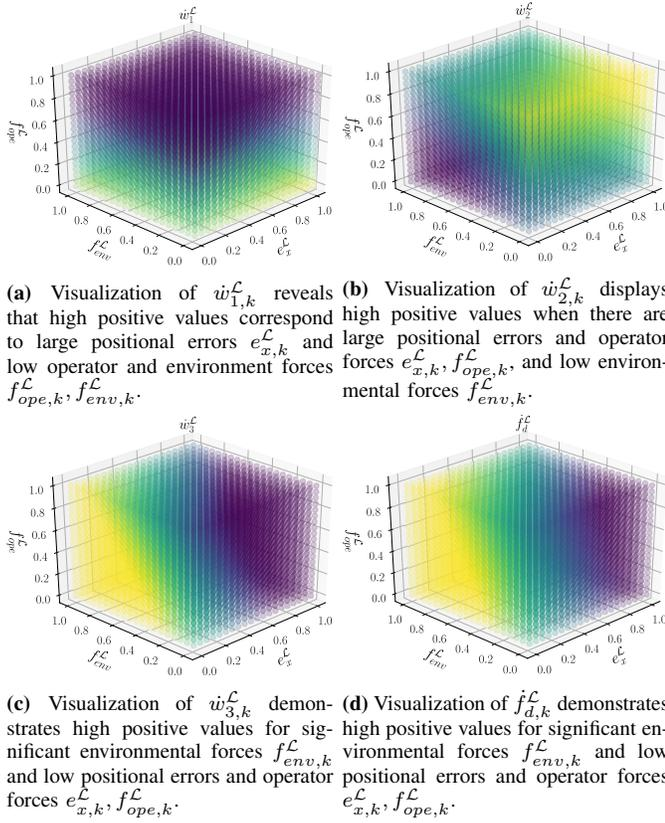
**Fig. 5:** Plot of the four action components  $a_k = \{\dot{w}_{1,k}^{\mathcal{L}}, \dot{w}_{2,k}^{\mathcal{L}}, \dot{w}_{3,k}^{\mathcal{L}}, \dot{f}_{d,k}^{\mathcal{L}}\}$  according to the three component of the state  $s_k = \{e_{x,k}^{\mathcal{L}}, f_{env,k}^{\mathcal{L}}, f_{ope,k}^{\mathcal{L}}\}$ . In this visualization, the color yellow indicates high positive rate of change values near 1, while the dark blue color represents high negative rate of change values near -1.
