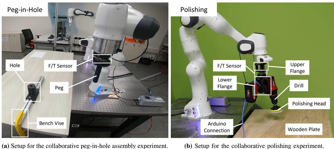
**Fig. 3:** The experimental setups. It is important to note that the operator must interact with the robot above the F/T sensor to prevent the misclassification of his interaction force  $\mathbf{f}_{ope}$  as the environment contact force  $\mathbf{f}_{env}$ .
