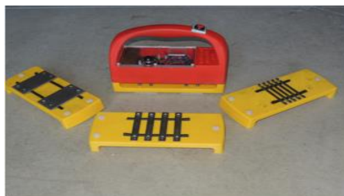
Figure 1: Capacitive plates and instrument developed by [8] and used for surface capacitive measurements.
