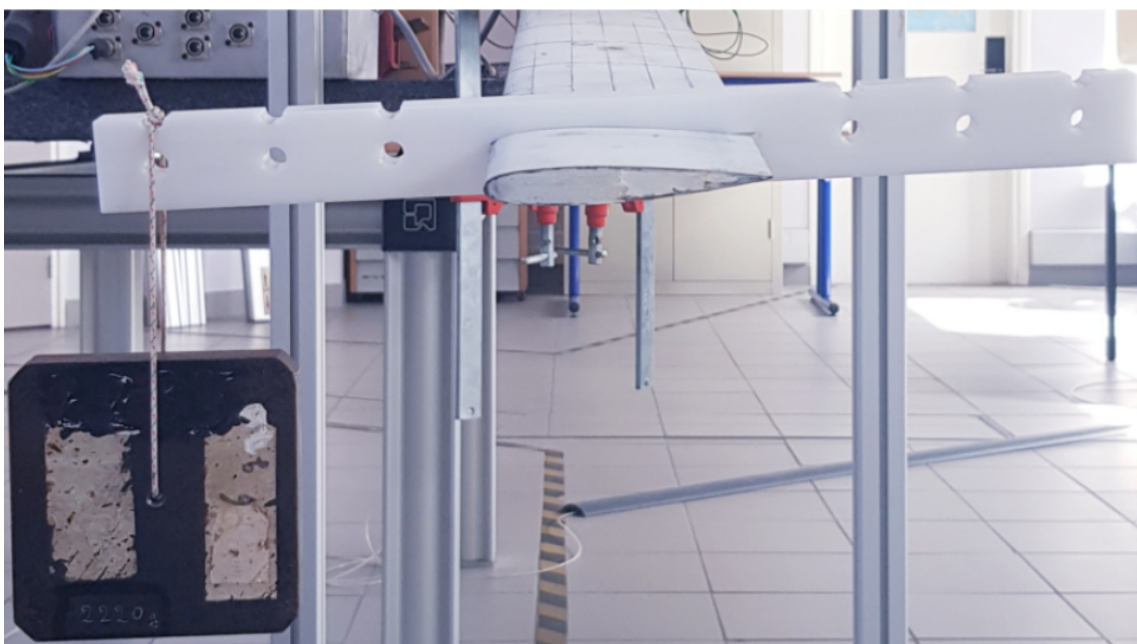
FIGURE 7: Experimental device used to study the mechanical properties of a foil [1]
