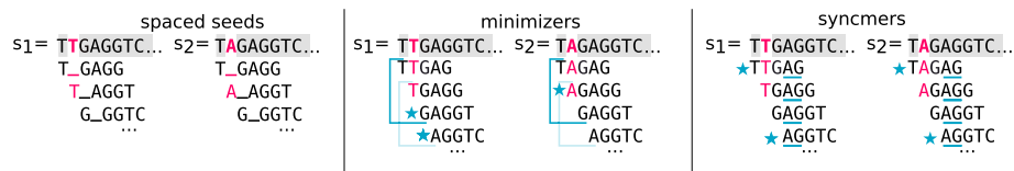
Fig. 3 Illustration of spaced-seeds, minimizer selection, syncmer selection and context dependency. Here, two sequences s_1 and s_2 are different from a single mutated base (second base, in pink). When comparing those sequences, one would like to focus on common bases, i.e., bases highlighted in grey. In the left panel, we present spaced-seeds for k = 5 , with a wildcard at second position (represented by an underscore). We observe that identical spaced-seeds can be spelled over a mutated locus, e.g., T_GAGG. In the middle panel, we present a selected minimizer with k = 5 , w = 3 . One blue window is presented, a second is suggested in lighter blue. A star shows the position of the selected k -mer in the window (we use lexicographic order). The mutated base has an impact on the overall window content, therefore a k -mer from the (unmutated) region of interest in s_1 is no longer selected in s_2 . On the contrary, in the right panel, we show that syncmers can be more robust in this situation. We choose k = 5 , s = 2 and present closed syncmers. We underline the smallest s -mer in each k -mer in blue and a star shows the selected k -mers. We see that in this example, the mutated base has no impact on the syncmer selection, and the same syncmer is selected in the region of interest for s_1 and s_2
