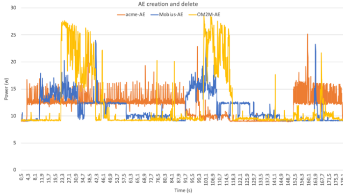
Fig. 8. Power consumption with the different IoT stacks for AE manipulation
