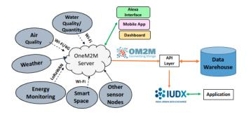
Fig. 2. OM2M based smart city deployment
