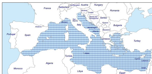
Figure 2. Sea mask used to calculate ozone averages over the Mediterranean (blue dots). The dots represent the grid cells considered in the averages.
