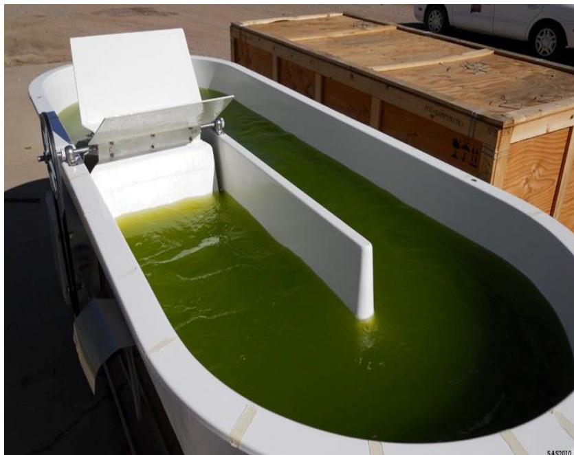
Open system fed with air (0.38% CO 2 )
