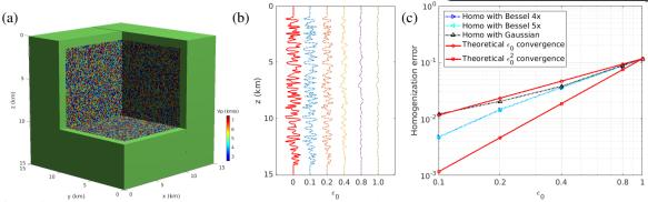
Figure 3 Homogenization test in a random medium. (a) The random P-wave velocity model  $V_p$ , (b)  $1D V_p$  profiles of the random model (red solid line) and the effective models using 4 Bessel filters with different  $\varepsilon_0$  (dash lines), (c) the convergence history of the wavefields generated from the effective models with respect to  $\varepsilon_0$  and the type of low-pass filters (Gaussian filter and its approximation through Bessel filters).
