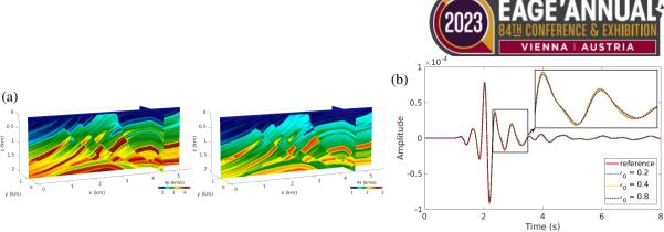
**Figure 4** (a) 3D Marmousi-II velocity models without the water layer which is used to calculate the reference solution for benchmarking against the homogenized solutions, (b) seismogram comparison of vertical displacement generated from (a) and the effective models with  $\varepsilon_0 = 0.2$ , 0.4 and 0.8 in Figure 5.
