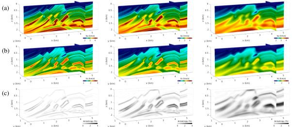
**Figure 5** 3D Marmousi-II effective models with  $\varepsilon_0 = 0.2$ , 0.4 and 0.8 from left to right. (a) P-wave velocity model  $(V_p)$ , (b) S-wave velocity model  $(V_s)$  and (c) the total anisotropy in percentage, which are calculated by projecting the resulting  $C_{ijkl}$  from homogenization to the closest isotropic model (Browaeys and Chevrot, 2004).
