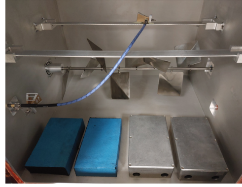
Fig. 6. Photograph of the two copies of the small shielded box #2 installed in the 0.580 \times 0.592 \times 0.595 \text{ m}^3 RC of IETR. The test configuration shown corresponds to the estimation of \sigma_{\text{abs\_out\_EUT}} ( Q_1 ).
