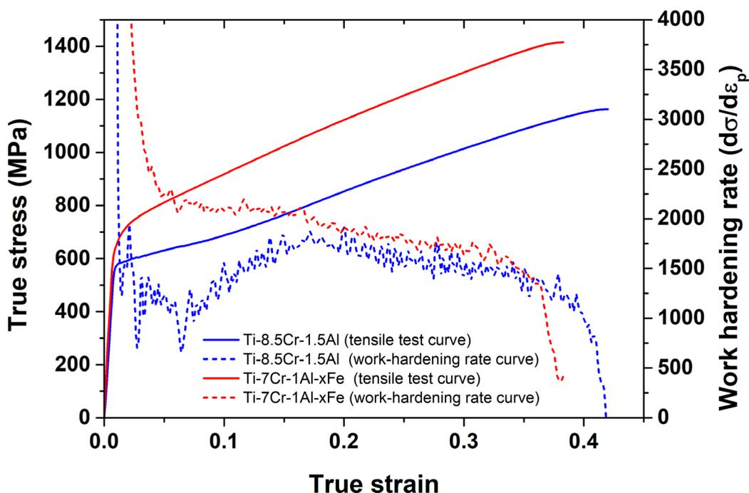
Figure 1 : Tensile true stress-true strain curve of Ti-8.5Cr-1.5Al (wt%) in blue and Ti-7Cr-1Al-xFe (wt%) in red, tested at room temperature at a strain rate of  $1.7 \times 10^{-3} \text{ s}^{-1}$ . Corresponding work-hardening rate curves as a function of true strain are plotted with dashed lines.
