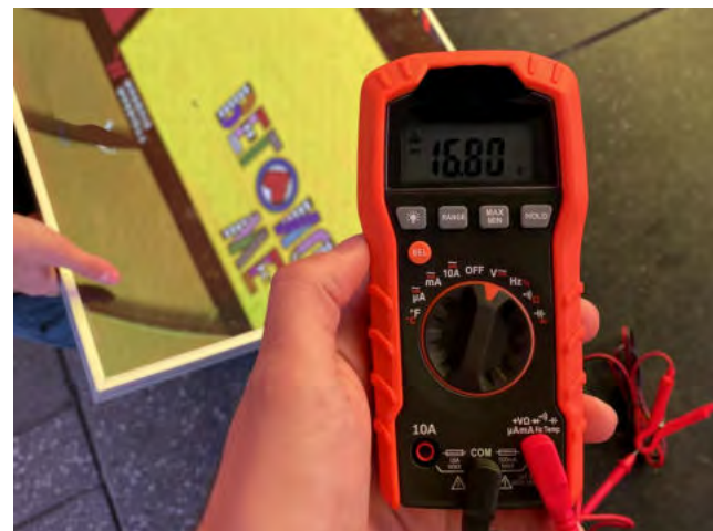
Figure 5: Voltage generated by photovoltaic cells tuned to a Times Square screen, Summer 2021. ©Present Authors.
