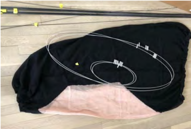
Figure 4 Knitted pink copper and polyester yarn with black cotton yarn, textile antenna material with compression frame rings and compressive fiberglass rods. © Felecia Davis, 2021
