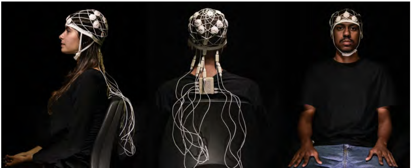
Figure 4. An EEG Schizocap , a cap composed of thirteen dry electrodes coupled to a crochet structure and connected to six EEG sensors and six corresponding channels of the BITalino microcontroller board, which digitizes and transmits the signals, via Bluetooth , to a computer running the data processing software. Photos: Thiago Barcelos. © 2018 by author
