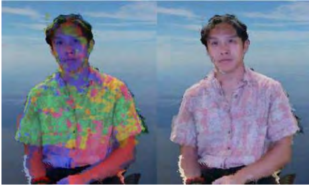
Figure 2. An example of the merged point clouds. On the left, the different colors each represent a view from one of the cameras.
