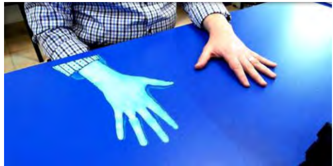
Figure 1: Our Possi(A)bilities system enables the experience of a video-projected virtual hand on the tabletop in front of a sitting user, where the virtual hand performs movements that are either synchronized with or decoupled from those of the physical hand next to it. By implementing a diversity of possi(a)bilities, e.g. , synchronized movements, delayed reaction time, or grasping with a smaller virtual hand, our system encourages reflection on the possible motor abilities of the human hand, readily observed by the user in real time.
