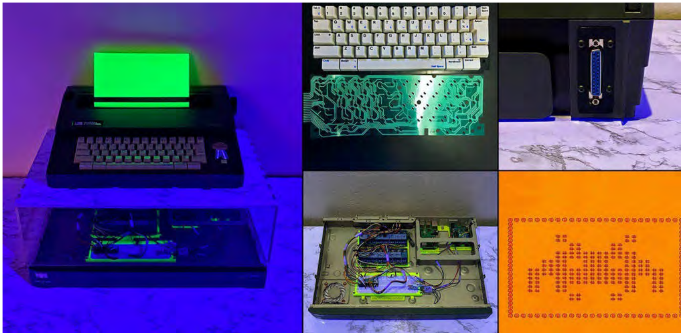
Figure 1: (Left) Exhibition of the Arduino AutoType at the Manetti Shrem Museum. (Upper-Center) The printed circuit board for the typewriter keyboard. (Upper-Right) the serial port that was added to the typewriter. (Bottom-Center) The Arduino AutoType Relay Module used to facilitate the communication between the typewriter and computer, note the blacklight sensitive labels on each module. (Bottom-Right) A sample print-out of the Arduino AutoType. ©Respect Copyright.
