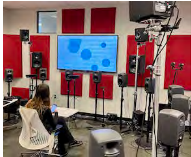
Figure 1. One of the authors demonstrating our smartphone-based, sound spatialization system in a simulated, multi-speaker laboratory environment.
