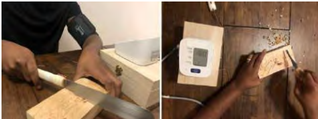
Figure 4. The Warming Saw warms the body during sawing and the Comfort-band Chisel tightens around the arm during chiseling.
