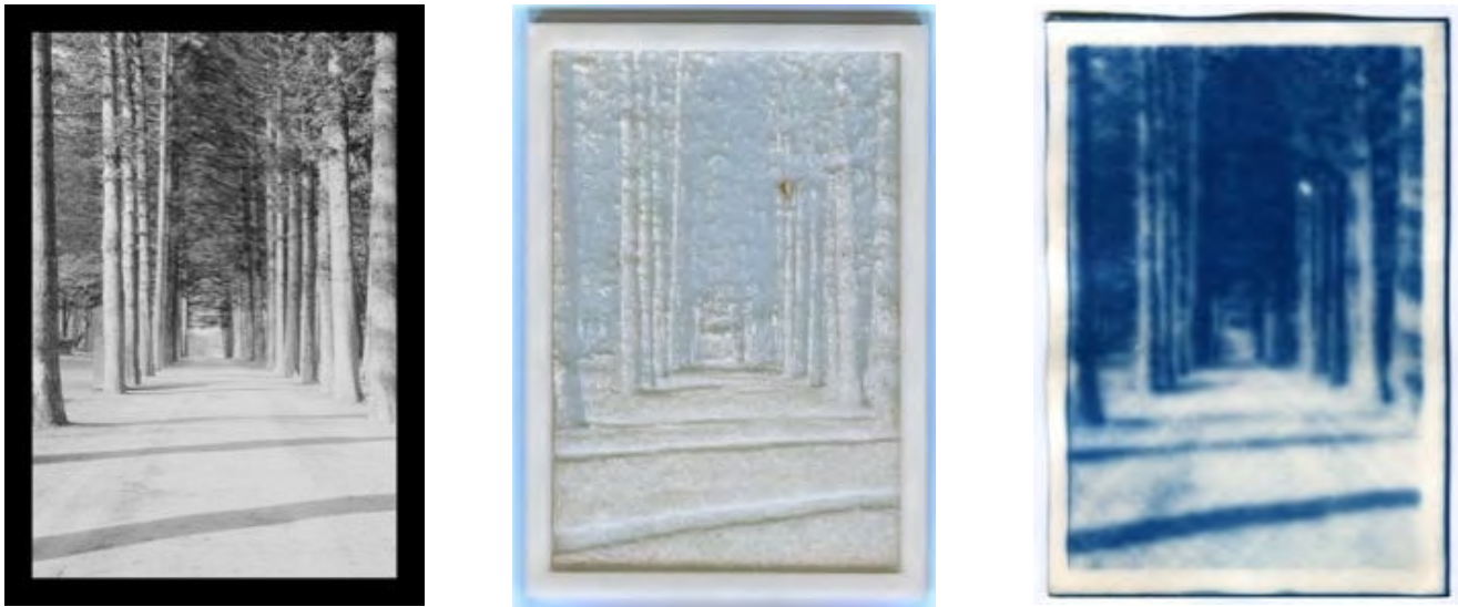
Figure 5 Image source for the test of the LUT (left), PLA stencil for the test print (middle), A cyanotype test print with the PLA stencil. (© the author. Photo: author)
