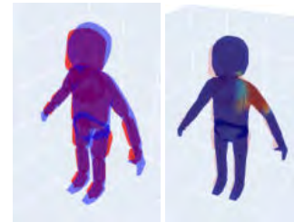
Figure 4: Armature and weights of ‘upper-arm.L’ bone automatically computed for a simple human figure
