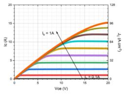
Fig. 15. On-state characteristic of the 5 mm  $\times$  5 mm electrical BJT shown in Fig. 12. The current gain reach 15.
