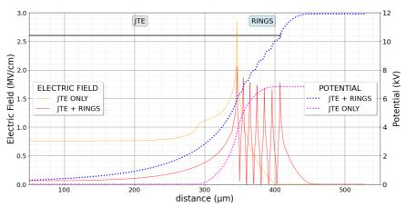
**Fig. 9.** Electric field and potential distribution over the horizontal axis through the peripheral protection as shown in Fig. 14.
