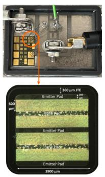
**Fig. 14.** Top: picture of a package with several dies to achieve high-current measurements. Bottom: picture of the bounded BJT die.
