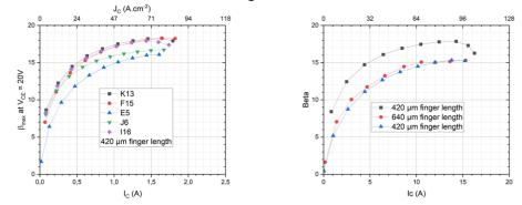
Fig. 16. Analysis of the current gain for various finger length of large electrical BJTs (5 mm × 5 mm) (a), analysis of the current gain for various small electrical BJT designs (1.4 mm × 1.4 mm) (b).
