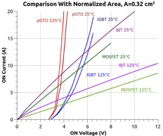
**Fig. 1.** I–V curve comparison of 15 kV SiC P-GTO, IGBT, and MOSFET at 25 °C and 125 °C [3] and our fabricated device 10 kV BJT (for  $I_B=1$  A).
