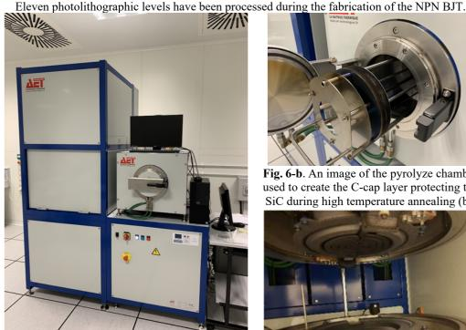
Fig. 6-a. AET furnace, utilized to activate the Al p-type doping created by ion implantation in the base and periphery (a).
