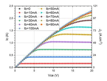
Fig. 13. Forward I-V characteristics of the fabricated BJT with an active area of 2.06 mm<sup>2</sup> measured on a probe station.
