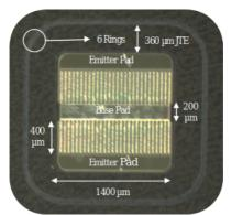
Fig. 3. Top microscopic view of 0.053 cm<sup>2</sup> fabricated BJT device with 2 emitter pads
