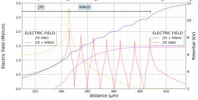
**Fig. 11.** Electric field and potential distribution over the horizontal axis cross section showing the uniform potential smoothing and optimal termination (Electric Field: red, Potential: blue) design and benefits against JTE only (Electric Field: orange, Potential: magenta).
