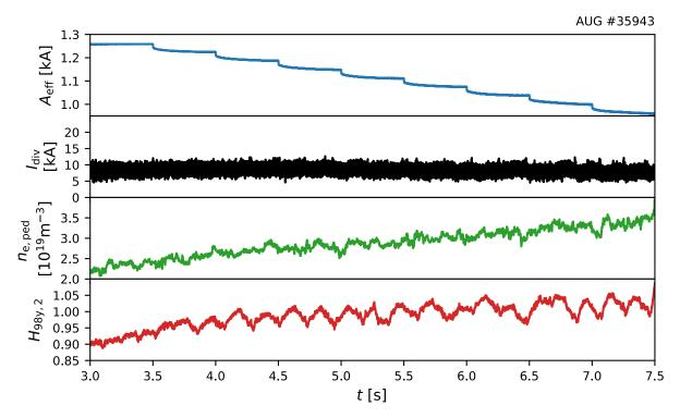
**Figure 4.** Time traces of AUG #35943 showing the effective coil current amplitude  $A_{\text{eff}}$ , the divertor shunt current  $I_{\text{div}}$ , the pedestal top electron density  $n_{\text{e,ped}}$  and the H-factor  $H_{98y,2}$ .
