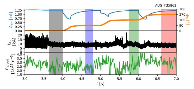
**Figure 21.** Time traces of discharge #35862 showing the effective RMP coil current amplitude  $A_{\text{eff}}$ , the toroidal orientation of the row of coils  $\Phi_0$ , the divertor shunt current measurement  $I_{\text{div}}$  and the electron density at the pedestal top  $n_{\text{e,ped}}$ . The colored and shaded time periods are the reference for figure 22.
