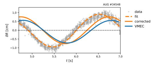
**Figure 7.** Time trace of the radial displacement of the density profile measured by the lithium beam diagnostic (grey dots), its fit (dashed orange line), its fit corrected for movements invoked by the plasma control system (solid orange line) and the VMEC prediction (solid blue) line during the rigid rotation in #34548.
