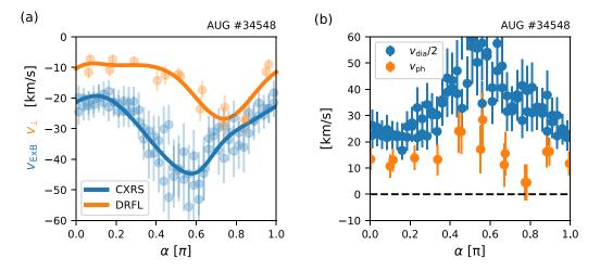
**Figure 19.** (*a*) Comparison between the minima of the ExB velocity  $v_{\text{ExB}}$  profiles (blue) and the perpendicular velocity  $v_{\perp}$  (orange) at the radial position of the  $E_r$  minimum tracked during the two rotation periods in #34548 as a function of the helical field line label  $\alpha$ . (*b*) Calculated phase velocity  $v_{\text{ph}}$  and half the ion diamagnetic velocity  $v_{\text{i,dia}}$  at the same radial position.
