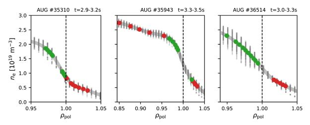
**Figure 20.** Electron density  $n_e$  profiles from three different ELM suppression discharges #35310, #35943 and #36514 as a function of the normalized poloidal flux coordinate  $\rho_{pol}$ . The dots mark the reflectometry measurement positions. Green (red) indicates that the QCM was (not) observed.
