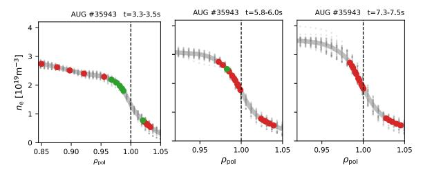
**Figure 5.** Electron density  $n_e$  profiles (combined lithium beam and Thomson scattering) taken at three different times during shot #35943 (see figure 4) as a function of the normalized poloidal flux coordinate  $\rho_{pol}$ . The dots mark the reflectometry measurement positions. Green (red) indicates that the QCM was (not) observed.
