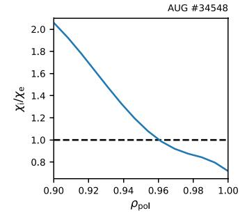
**Figure 24.** Radial profile of the ratio of ion  $\chi_i$  to electron  $\chi_e$  heat conductivity as calculated from power balance.
