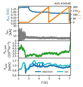
**Figure 6.** Time traces of the toroidal RMP orientation variation in shot #34548, showing the effective RMP coil current amplitude  $A_{\text{eff}}$  and toroidal orientation of the upper row of  $\text{coils}\Phi_0$ , the divertor shunt current  $I_{\text{div}}$ , the electron density at the pedestal top  $n_{\text{e,ped}}$ , as well as the electron  $T_{\text{e,ped}}$  and ion  $T_{\text{i,ped}}$  temperatures close to the pedestal top.
