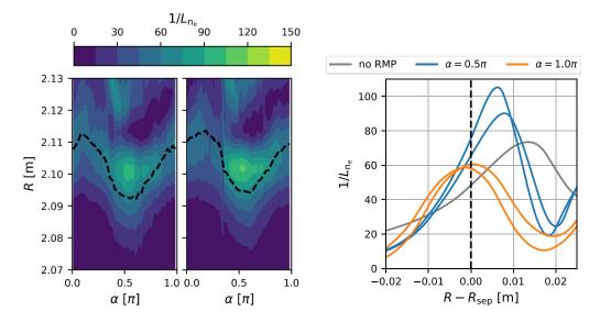
**Figure 15.** Left: contour plot of the inverse gradient length of the electron density (lithium beam) as a function of the radial position *R* and helical field line label  $\alpha$  during both rotation periods in #34548. Here,  $\alpha$  is always calculated just inside the separatrix. Right: comparison of profiles inside (blue) and outside (orange) the fluctuation gap to the reference case without RMPs (grey) of shot #33 998 at t = 2.8-3.1 s.
