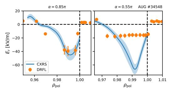
**Figure 18.** Radial profiles of the radial electric field measured by CXRS (blue) and DRFL (orange) in #34548. Profiles are compared for for  $\alpha = 0.85 \pi$  (left) and  $\alpha = 0.55 \pi$  (right). The vertical and horizontal dashed lines indicate the separatrix and  $E_r = 0$ , respectively.
