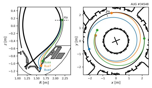
**Figure 14.** Poloidal cross-section (left) and top-down view (right) showing the field line tracing from 3 exemplary divertor Langmuir probes to the horizontal plane of the perpendicular reflectometry Ka-band antenna.
