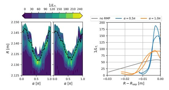
**Figure 16.** Left: contour plot of the inverse gradient length of the ion temperature (CXRS) as a function of the radial position *R* and helical field line label  $\alpha$  during both rotation periods in #34548. Here,  $\alpha$  is always calculated just inside the separatrix. In the white area no measurements are available. Right: comparison of profiles inside (blue) and outside (orange) the fluctuation gap to the reference case without RMPs (grey) of shot #33 998 at t = 2.8-3.1 s.
