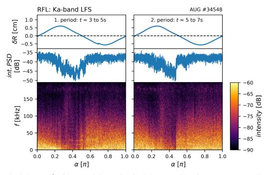
**Figure 8.** The radial displacement  $\delta R$  of the separatrix intersecting with the beam path of the reflectometer, the measured integrated power spectral density PSD and its spectrogram for the Ka-band reflectometry system (37 GHz probing frequency) on the LFS as a function of the helical field-line label  $\alpha$  for both rotation periods of AUG #34548.
