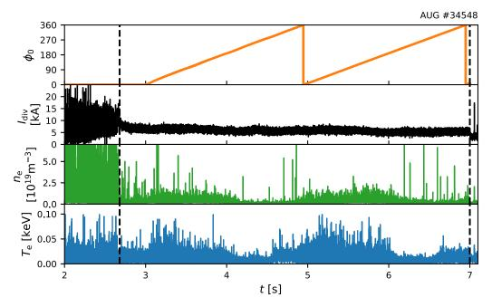
**Figure 11.** Time traces of the toroidal orientation of the upper row of coils  $\phi_0$ , the divertor shunt current  $I_{\text{div}}$  as well as the electron density and temperature measured by Langmuir probe 8ua7 in #34548. ELMs are suppressed in between the two dashed lines.
