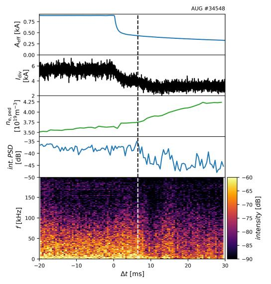
**Figure 2.** Time traces of AUG #34548 showing the effective RMP coil current amplitude  $A_{\text{eff}}$ , the divertor shunt current  $I_{\text{div}}$ , the electron density at the pedestal top  $n_{\text{e,ped}}$ , the integrated power spectral density *PSD*, and the spectrogram of the reflectometry measurement with a probing frequency of 37 GHz. The dashed line indicates the onset of the decay of the spectral density simultaneous with a further decrease of the  $I_{\text{div}}$  baseline.
