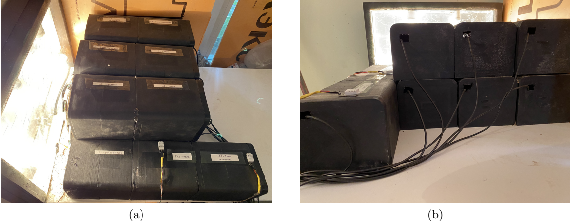
Figure 4. Containers with different soils (a), container's backside with sensor cables (b).
