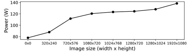
Figure 3: Average node power consumption as a function of the frames size ( $0 \times 0$  represents the idle power consumption of the VLC server).
