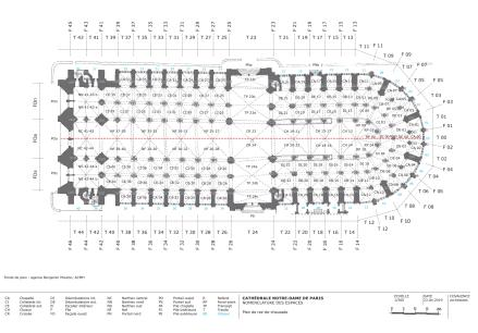
**Figure 1:** Plan of the ground floor of the cathedral with the nomenclature entities as defined by the architects of the restoration project (@RNDP).
