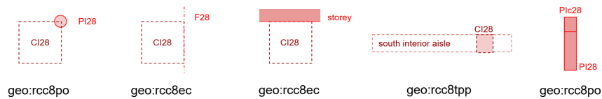
Figure 7: Array of spatial relations expressed using the geoSPARQL RCC8 model between heterogeneous spatial entities with the example presented in [Figure 6] and [Table 2]
