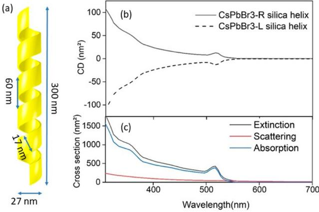
**Figure 3.** (a) Dimension of the PNC helix used for the simulation. (b) Simulated circular dichroism of H-PNCs. (c) Extinction, absorption, and scattering cross sections of H-PNC simulated by the boundary element method for unpolarized incident light.
