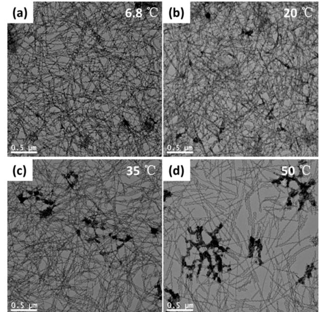
**Figure 5.** Lower magnification of TEM images of PNC growth at 6.8 °C (a), 20 °C (b), 35 °C (c), and 50 °C (d), respectively.
