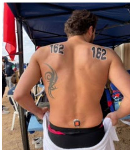
150 Figure 1. IMU location on the sacrum of the swimmer.
