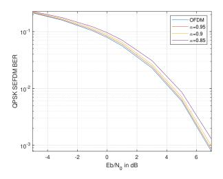
Fig. 7. Comparison of BER of uncoded SEFDM with OFDM for QPSK modulation and  ${\cal N}=24$
