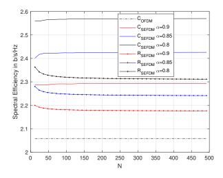
Fig. 3. Capacity and rate comparison between SEFDM and OFDM for N=48
