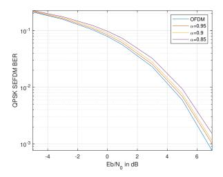
Fig. 10. Comparison of BER of uncoded SEFDM with OFDM for QPSK modulation and  ${\cal N}=60.$
