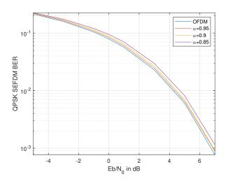
Fig. 6. Comparison of BER of uncoded SEFDM with OFDM for QPSK modulation and  $N=12\,$
