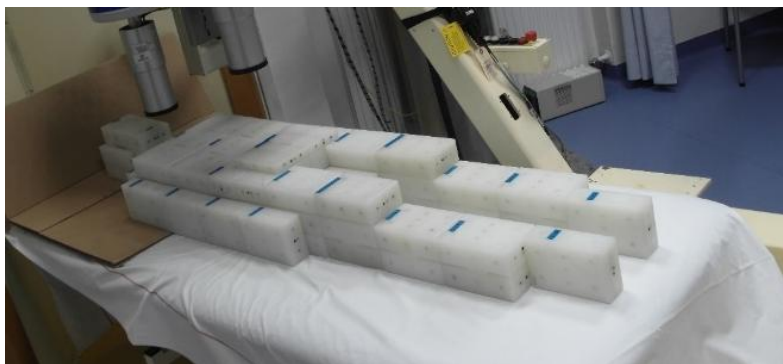
Fig 2 Photo of the phantom in the P4/70 kg configuration, erected in a whole-body counter with stretcher geometry.
